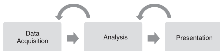
Figure 1.1 Virtual instrumentation model.
